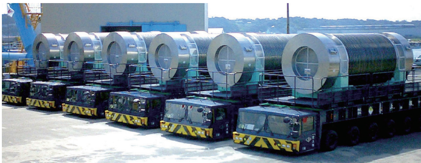
Speed Carrier (140 tons)
