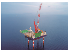
"CP-8001" Multipurpose Self-Elevating Platform
