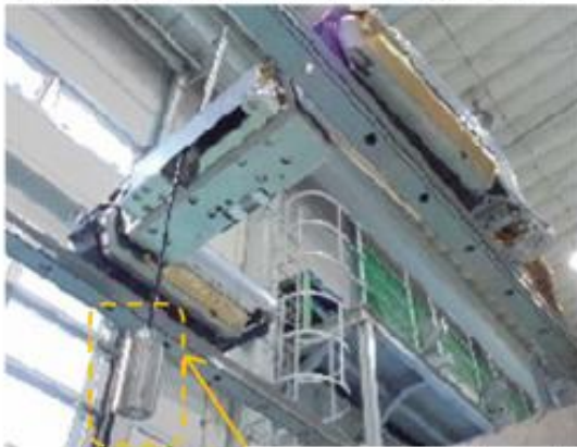
Sensor unit integrating a camera and dosimeter
